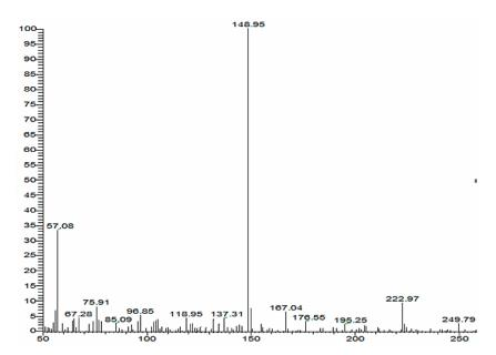
**Figure 2.** The spectrum of the isolated peak, got when analysing the aqueous extract from the medium plasticized PVC material (extraction at 70 °C). X-axis: the ratio of the mass of the ion to its charge. Y-axis: the relative amount of ions of the given species
